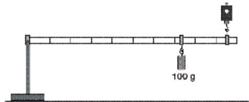
1. Determine the mass of the meter stick and record the value in data table 1 on page 4
