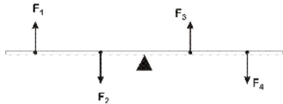
Our convention is that we will label torques that would tend to rotate the object counter clockwise as positive. Torques that would tend to make the object rotate clockwise we will label as negative.
