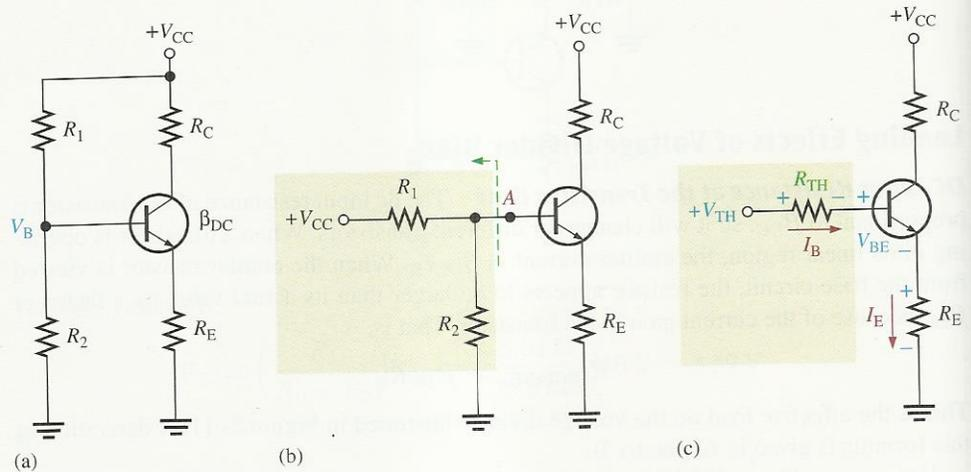
The Thevenin equivalent of the bias circuit, connected to the transistor base, is shown in the beige box in Figure 5-13(c). Applying Kirchhoff's voltage law around the equivalent base-emitter loop gives
