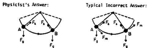
Fig. 1. Correct and incorrect answers to pendulum problem.
