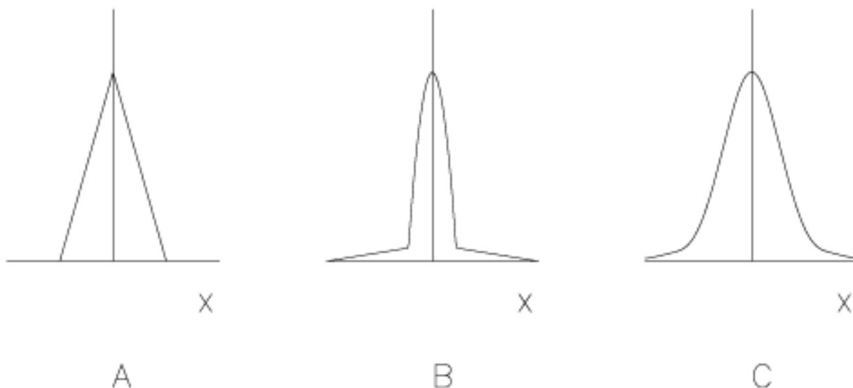
Figure 3: The  $x$ -axis is position along the scan direction and the  $y$ -axis is the count rate. Panel A shows the response to an isotropically radiating source. The width of the base is 0.4 cm is the width of the slit. Panel B shows the distribution of gamma rays from the source. Panel C shows the convolution of these 2 responses.
