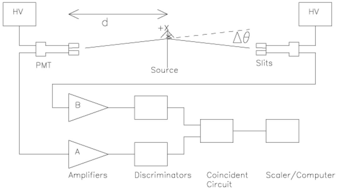
Figure 1: Block diagram of the positron annihilation experiment. The source is at the asterisk. HV stands for the high voltage supply and PMT stands for the photomultiplier tube.
