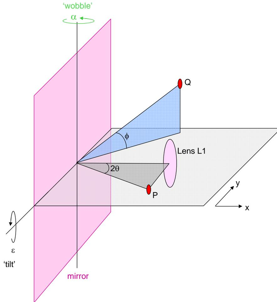
Figure 8: Geometry for illuminating the MSE plasma-facing lens.
