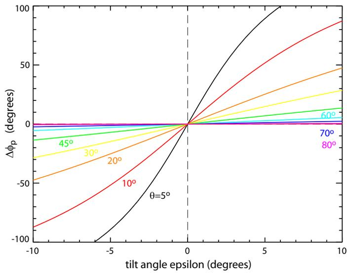
Figure 9: Change in polarization angle upon reflection from a perfect dielectric mirror for the simplified ‘tilt’ geometry ( $\phi = \alpha = 0$ ) as a function of the tilt angle  $\epsilon$  and the angle-of-incidence  $\theta$ .
