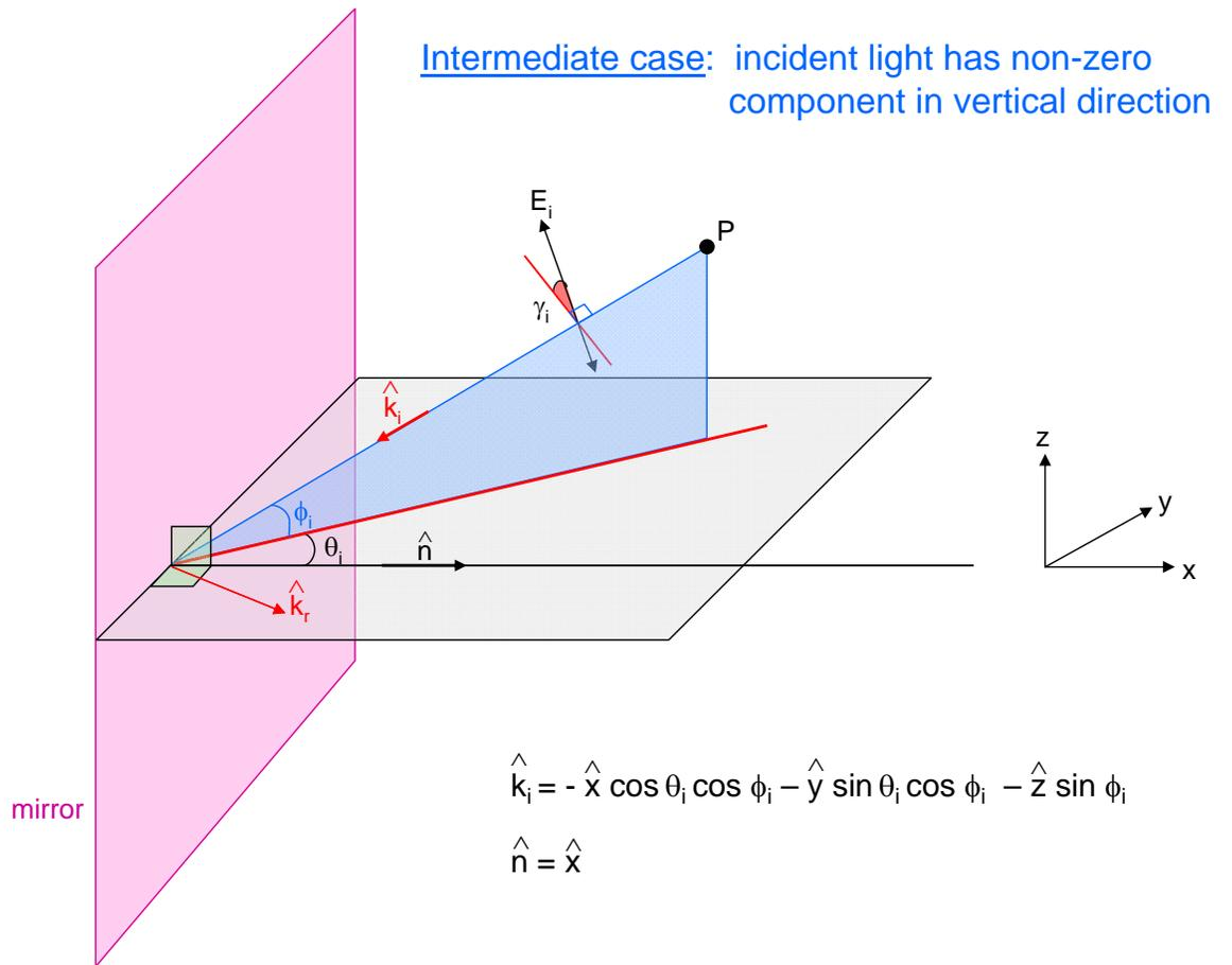
Figure 5: Geometry for computing the polarization upon reflection from an ideal, flat mirror. For this case, the  $k$ -vector of the incident light is allowed to have a non-zero component in the  $z$  - direction, but the mirror normal is still assumed to be in the  $\hat{x}$  direction.
