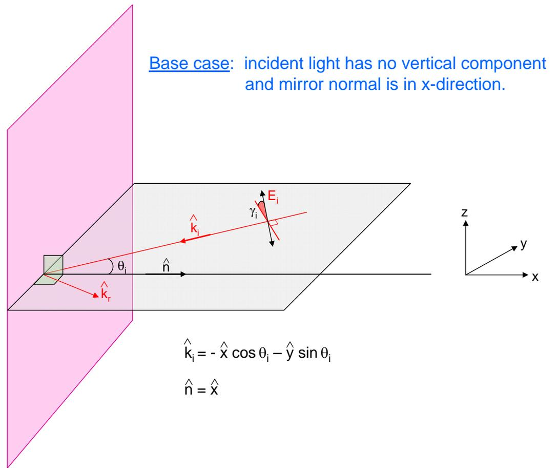
Figure 4: Geometry for computing the polarization upon reflection from an ideal, flat mirror. For this case, the  $k$ -vector of the incident light is assumed to lie in the  $x - y$  plane, and the mirror normal is assumed to be in the  $\hat{x}$  direction.
