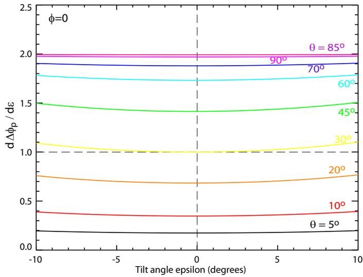
Figure 12: Absolute value of the rate-of-change of polarization angle as tilt angle is varied,  $dD\phi_p/d\epsilon$  upon reflection from a perfect metal mirror for the simplified ‘tilt’ geometry ( $\phi = \alpha = 0$ ) as a function of the tilt angle  $\epsilon$  and the angle-of-incidence  $\theta$ .
