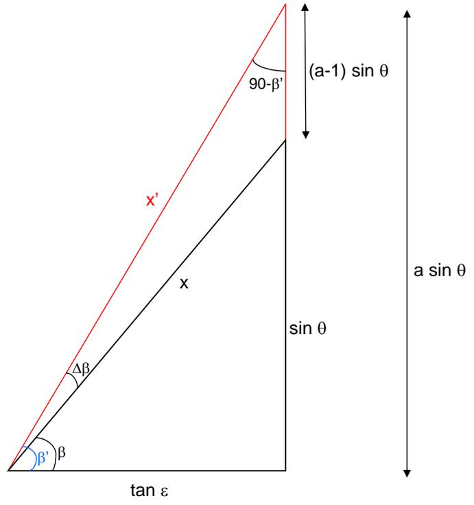
Figure 7: Geometry for computing the change in polarization angle.
