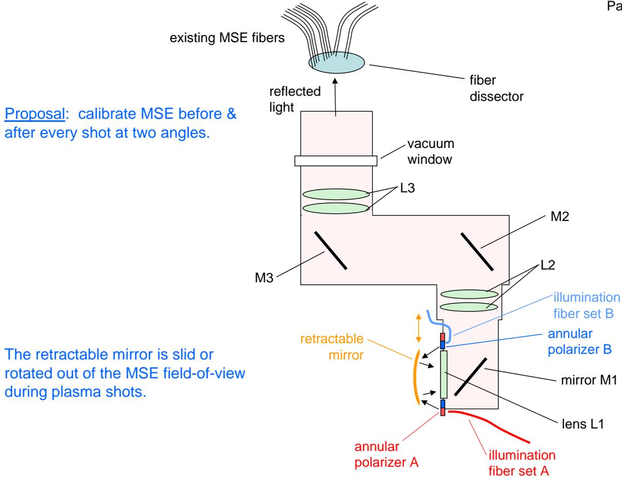
Figure 2: Proposed system for an in-situ calibration system for MSE on Alcator sc c-mod. Linearly polarized light strikes a mirror that is slid in front of the plasma-facing lens shortly after a shot.
