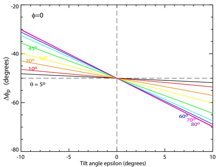
Figure 11: Change in polarization angle upon reflection from a perfect metal mirror for the simplified ‘tilt’ geometry ( $\phi = \alpha = 0$ ) as a function of the tilt angle  $\epsilon$  and the angle-of-incidence  $\theta$ . For these calculations the input polarization angle  $\phi_p = 25^\circ$ .
