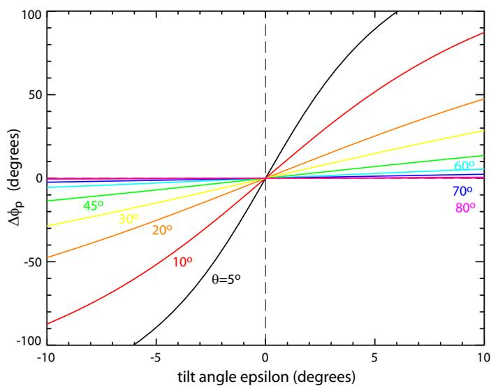
Figure 10: Absolute value of the rate-of-change of polarization angle as tilt angle is varied,  $dD\phi_p/d\epsilon$  upon reflection from a perfect dielectric mirror for the simplified ‘tilt’ geometry ( $\phi = \alpha = 0$ ) as a function of the tilt angle  $\epsilon$  and the angle-of-incidence  $\theta$ .
