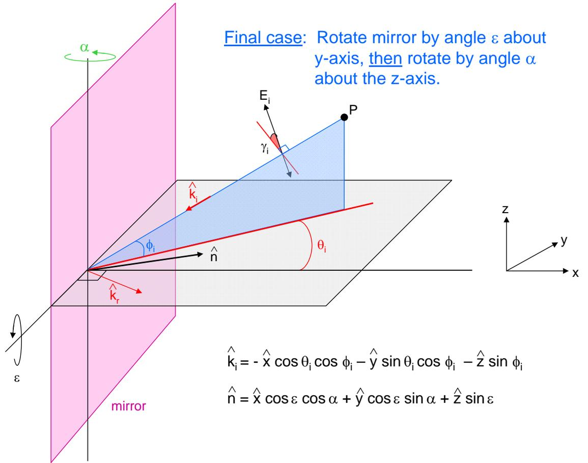
Figure 6: Geometry for computing the polarization upon reflection from an ideal, flat mirror. For this case, the  $k$ -vector of the incident light is allowed to have a non-zero component in the  $z$  - direction. The mirror is rotated an angle  $\varepsilon$  about the  $y$ -axis and then the mirror is rotated by an angle  $\alpha$  about the  $z$ -axis.
