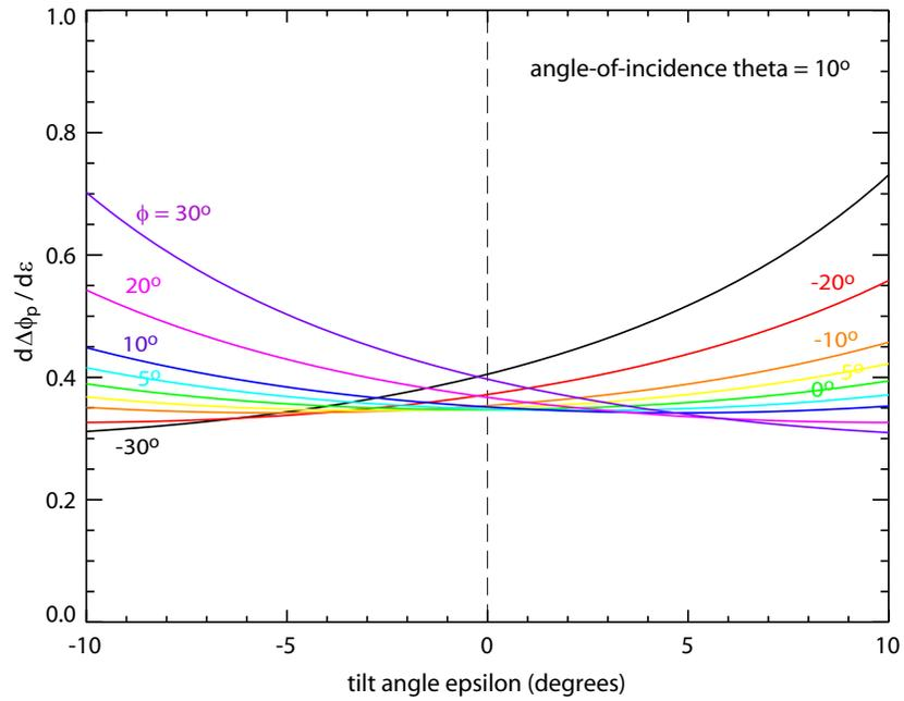
Figure 14: Absolute value of the rate-of-change in polarization angle as the tilt angle is varied,  $dD\phi_p/d\epsilon$  upon reflection from a perfect metal mirror for an angle-of-incidence  $\theta = 10^\circ$  as a function of the ‘elevation angle’  $\phi$  and the tilt angle  $\epsilon$ . For these calculations the input polarization angle  $\phi_p = 25^\circ$ .
