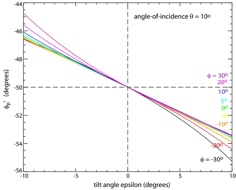
Figure 13: Change in polarization angle upon reflection from a perfect metal mirror for an angle-of-incidence  $\theta = 10^\circ$  as a function of the ‘elevation angle’  $\phi$  and the tilt angle  $\epsilon$ . For these calculations the input polarization angle  $\phi_p = 25^\circ$ .
