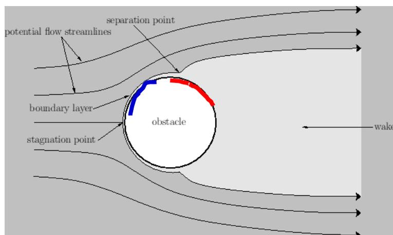
These molecules in this boundary layer collide with incoming particles just slightly above, slowing those down and inducing the flow to rotate (the molecules to tumble over each other). These molecules, in turn, also slow down the flow just above them. Higher above the surface the molecules are more affected by the fast flowing air, and not by the ball.
