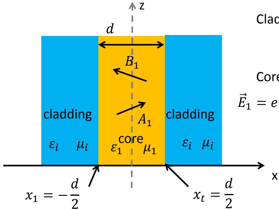
Cladding:  $\vec{E}_i = A_i e^{j(\omega t - \beta z)} e^{\kappa_{ix}(x - x_1)} \vec{e}_y$
