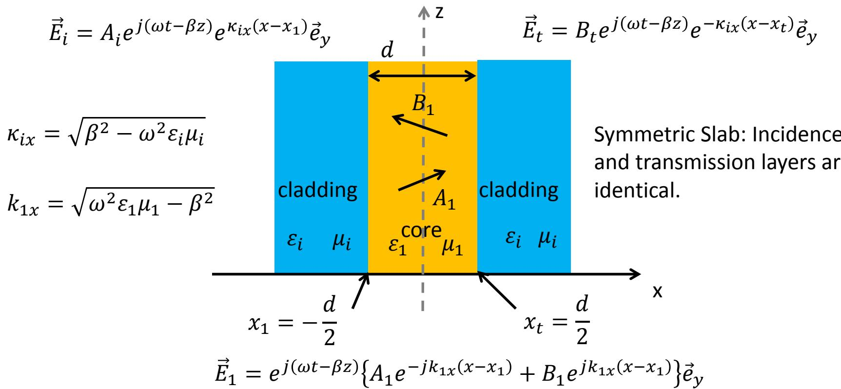
Due to the symmetry of the waveguide geometry, the electric field in the core region can be expressed as either a sin or a cos function.
