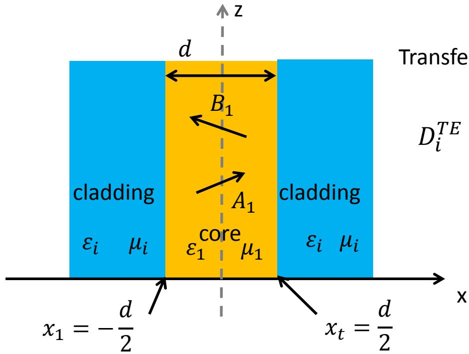
Transfer matrix between the cladding and core layer:
