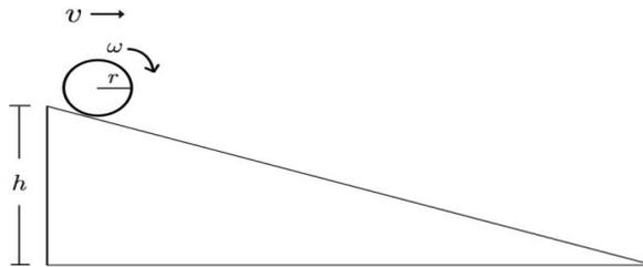
*Figure 3. Illustration of the initial position of the cylindrical shell and its intended trajectory along the inclined plane*
