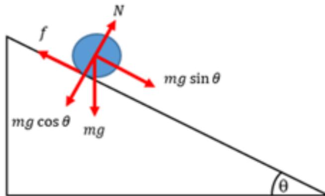
*Figure 2. Illustration of the forces acting on the center of mass of the fluid-filled hollow cylindrical shell*
