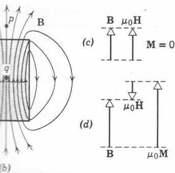
lines of **B** for a permanent magnet. The boundary. The closed dashed Ampère's law may be applied. The for (c) a particular outside point *p*
