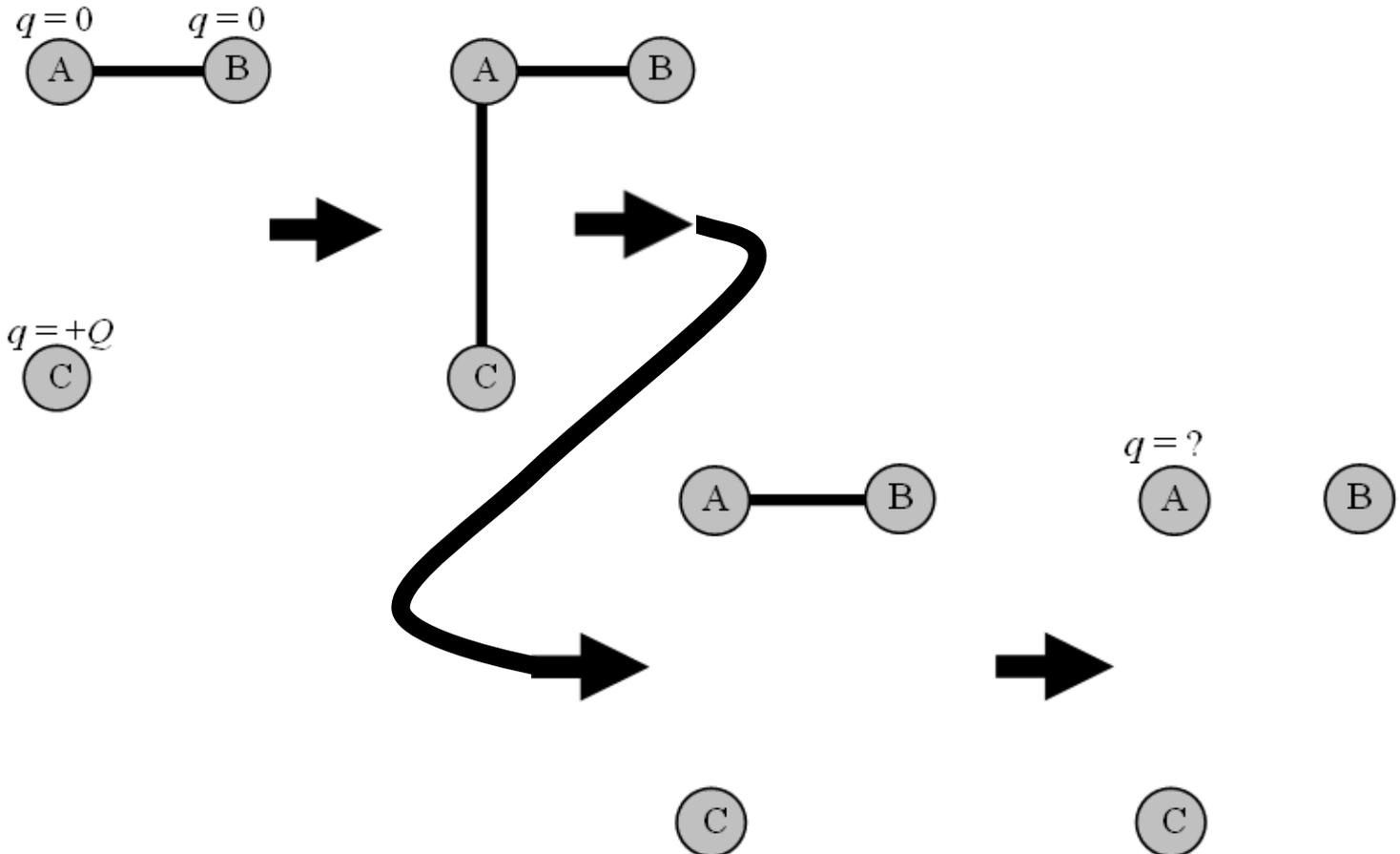
18.4.5. Consider the conducting spheres labeled A, B, and C shown in the drawing. The spheres are initially charged as shown on the left, then wires are connected and disconnected in a sequence shown moving toward the right. What is the final charge on sphere C at the end of the sequence?
