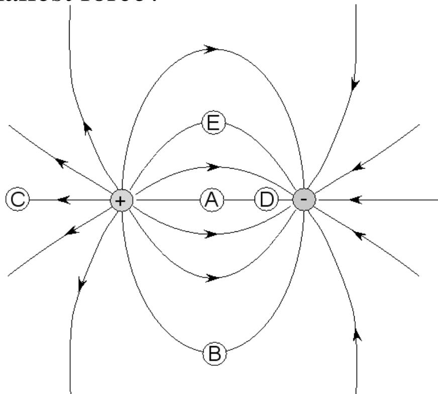
18.7.10. A positively charged object is located to the left of a negatively charged object as shown. Electric field lines are shown connecting the two objects. The five points on the electric field lines are labeled A, B, C, D, and E. At which one of these points would a test charge experience the largest force?
