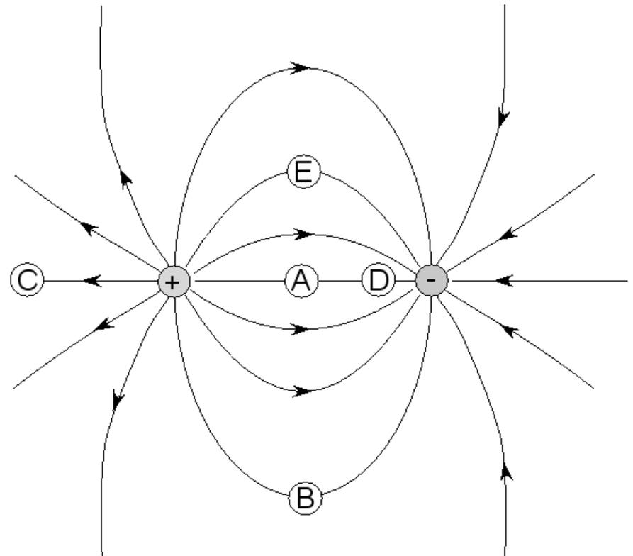
18.7.9. A positively charged object is located to the left of a negatively charged object as shown. Electric field lines are shown connecting the two objects. The five points on the electric field lines are labeled A, B, C, D, and E. At which one of these points would a test charge experience the smallest force?
