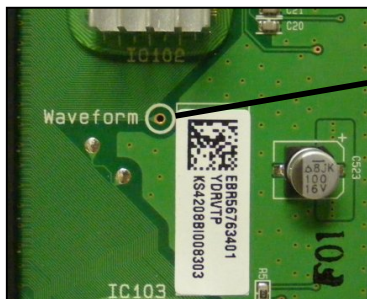
Y-Drive Board Test Point
