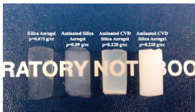
**FIGURE 1.** Transparent silica aerogel and aminated silica aerogel. After CVD of methyl cyanoacrylate, the gels begin to become opaque.
