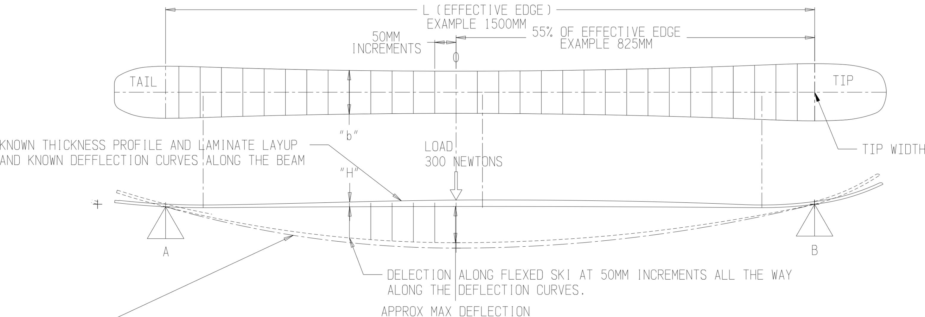
KNOWN THICKNESS PROFILE AND LAMINATE LAYUP AND KNOWN DEFFLECTION CURVES ALONG THE BEAM
